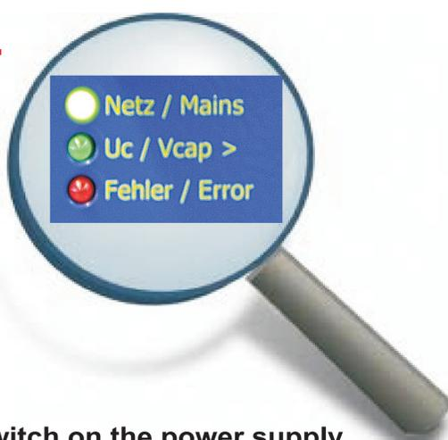
Switch on the power supply. The C-TEC P is charging. The LED „Netz/Mains“ illuminate
