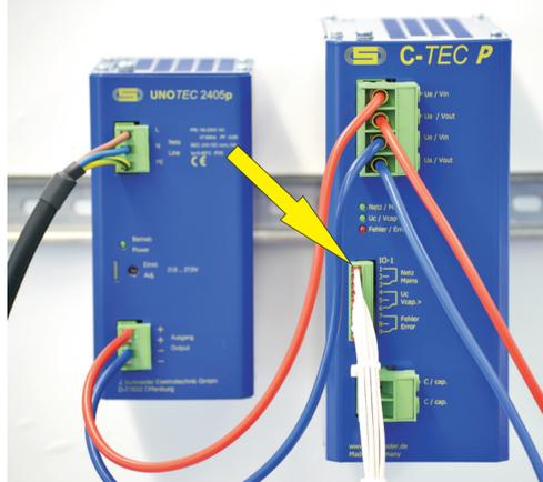
Wiring of the inputs/outputs
