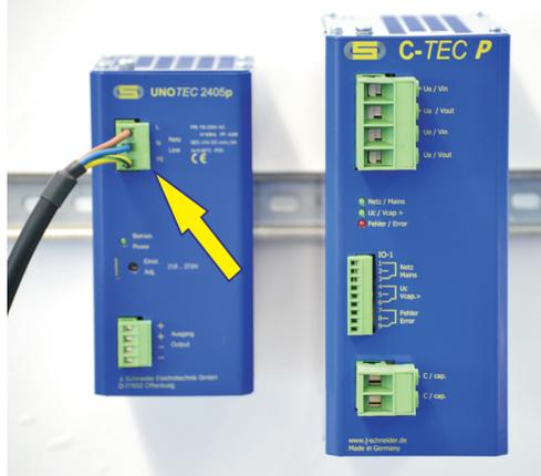
Connect the 24 V DC power supply to the mains (230 V AC)
