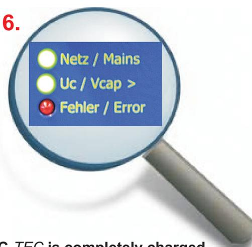
C-TEC is completely charged. The LEDs „Netz/Mains“ and „U<sub>C</sub>/V<sub>cap</sub> >“ illuminate
