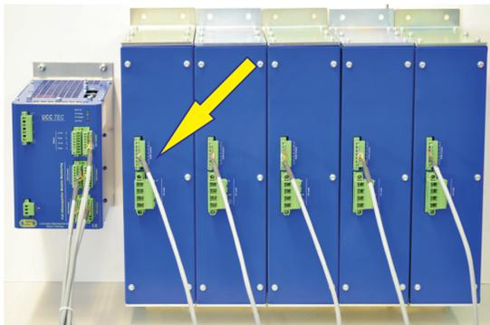
Connection data line from UCC-TEC to the UC-moduls
