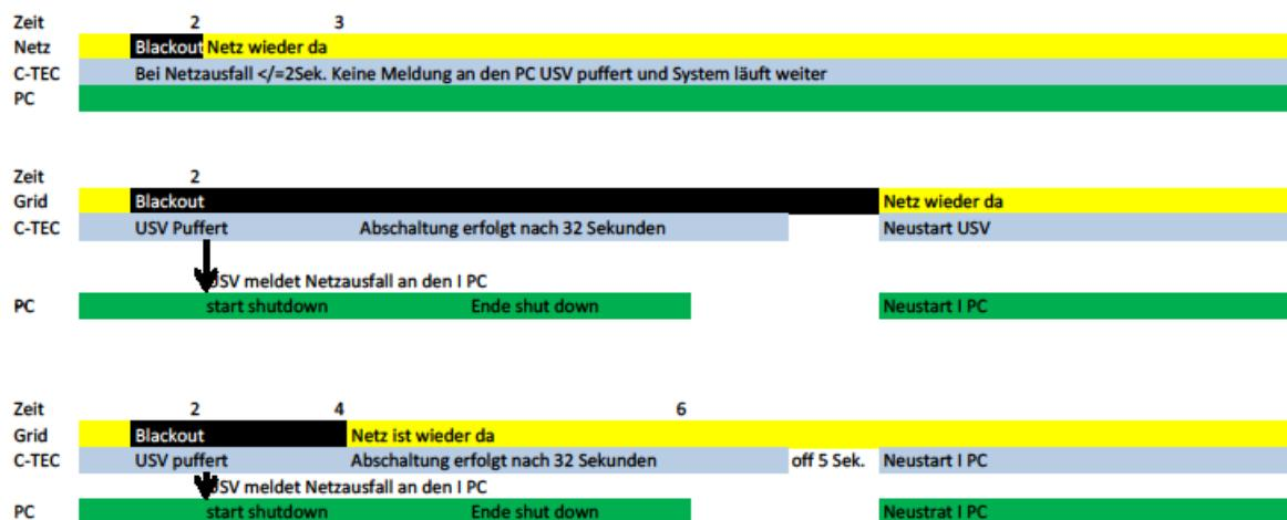
**CAUTION:** if the mains failure is > 2 seconds, the **C-TEC** switches off at the latest 40 seconds afterwards for at least 5 seconds.
