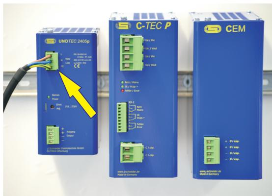
Connect the 24 V DC power supply to the mains (230 V AC)
