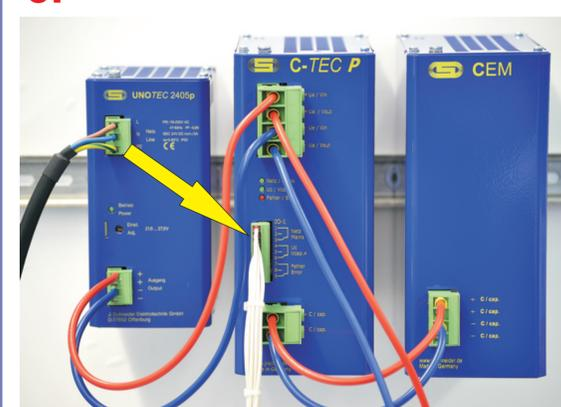
Wiring of the inputs/outputs
