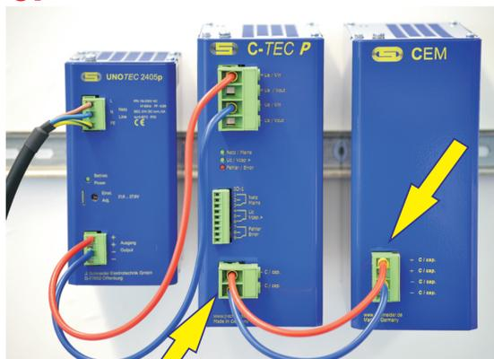
Connect the CEM to the capacitor output of the C-TEC P
