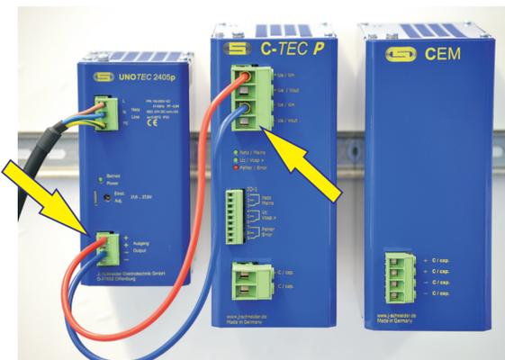
Connect the C-TEC P to the output of 24 V DC power supply
