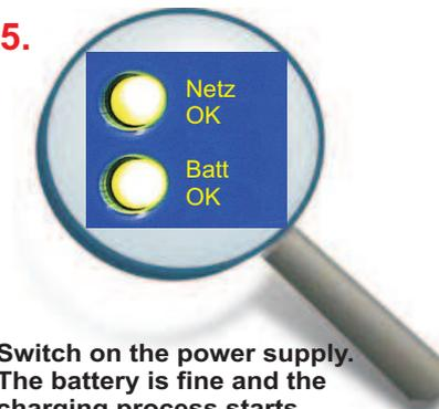
Switch on the power supply. The battery is fine and the charging process starts. The LEDs „Netz OK“ and „Batt OK“ illuminate
